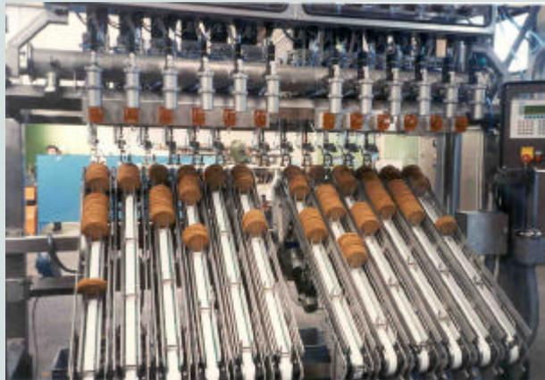
In the equipment's construction have been used the hygiene and cleanability criteria typical of the alimentary industry; in particular design and realization have been executed to exclude weldings and plane surfaces on which dirty could deposit.
