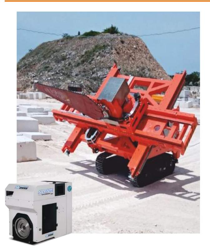
HYBRID MACHINE THIS VERSION IS ALSO EQUIPPED WITH A DIESEL ENGINE THAT ALLOWS THE MACHINE TO MOVE BY ITSELF WITH TRACKS
