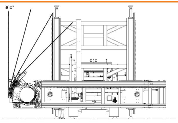
THE HEAD, IN THIS NEW CONCEPT, IS FIXED ON A COMPACT TROLLEY WHICH ENCLOSES THE SLIDING SYSTEM AND THE HEAD'S FIFTH WHEEL,
