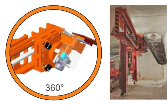
FIXING BY THE OPERATOR THE MECHANICAL LOCKS (6 BOLTS) ARE NO LONGER NEEDED *TIME SAVING/INCREASE SAFETY* IT CAN TURN 360° IN ANY POSITION, WITHOUT INTERLOCKS *SPEED-UP THE PROCESS* NOW, IT TURNS ONLY THE HEAD, LIGHTEN THE LOAD ON THE FRAME *LESS STRESS FOR THE FRAME AND GEARBOXES*
