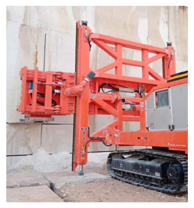
BEING ENGINEERED TO PERFORM A COMPLETE TUNNEL ADVANCEMENT WITH ONLY ONE POSITIONING, THE FRAME HAS BEEN STRENGTHENED
