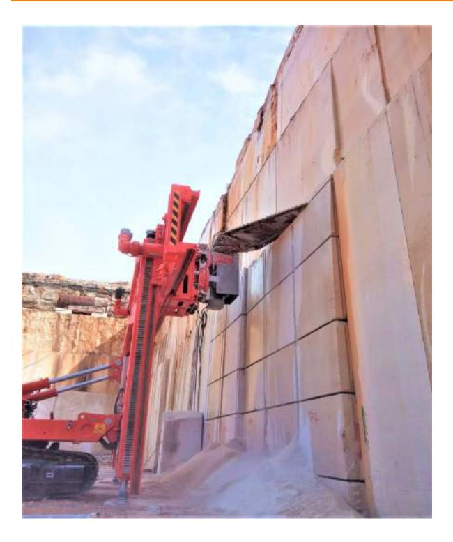
100% ELECTRIC MACHINE MOST OF THE MOVEMENTS AND ALL THE CUTTING UTILITIES AS CHAIN ROTATION, ARM ROTATION, TRANSLATION ARE POWERED BY ONLY ELECTRIC MOTORS
